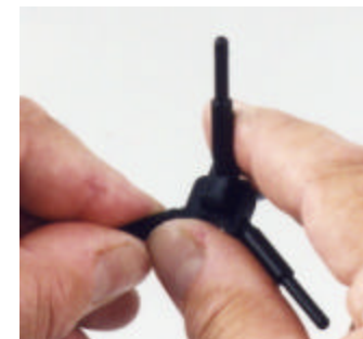
Figure 4. Disassembling the tetrahedral atom This may be accomplished in one motion with One hand, by placing two or four fingers across the “V” slightly and push the two pieces apart. In Figure 4, the left hand stabilizes the piece while the right hand spreads both pieces and separates them.
